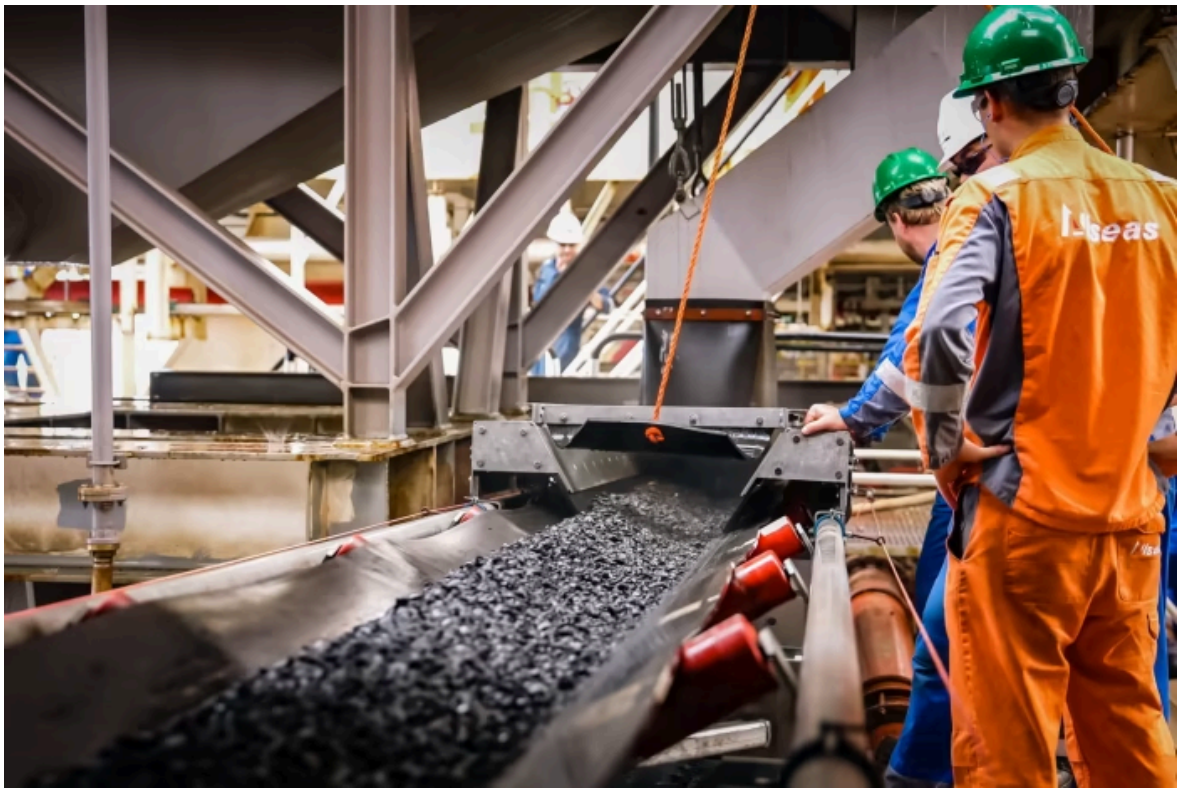
Engineers inspect the first batch of polymetallic nodules collected from the sea floor during TMC's trial last November © Richard Baron/The Metals Company
